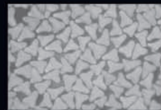
Triangle cross section and bright polymer fiber with shiny appearance like silk and unique touching
